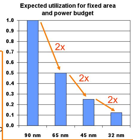
Utilization Wall: With each successive process generation, the percentage of a chip that can actively switch drops exponentially due to power constraints.
