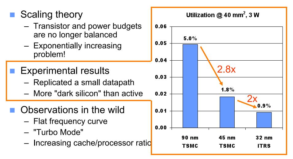
Utilization Wall: With each successive process generation, the percentage of a chip that can actively switch drops exponentially due to power constraints.
