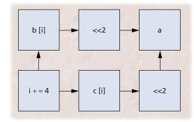
Figure 3. Six-tile systolic structure that maintains value dependencies for a looped array access.
