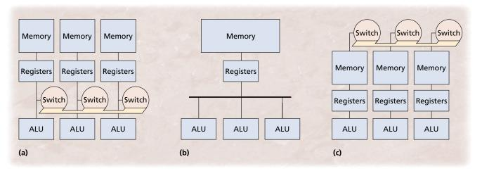
Figure 2. Raw microprocessors differ from superscalar and multiprocessor architectures. (a) Raw microprocessors distribute the register file and memory ports and communicate between ALUs on a switched, point-to-point interconnect. (b) A superscalar contains a single register file and memory port and communicates between ALUs on a global bus. (c) Multiprocessors communicate at a much coarser grain through the memory subsystem.
