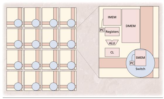
Figure 1. A Raw processor is constructed of multiple identical tiles. Each tile contains instruction memory (IMEM), data memories (DMEM), an arithmetic logic unit (ALU), registers, configurable logic (CL), and a programmable switch with its associated instruction memory (SMEM).
