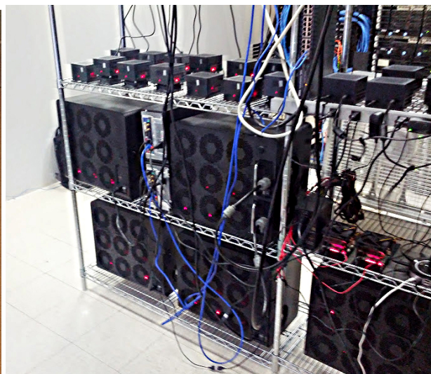
Figure 7: Newly arrived $22,484 65-nm ASIC-based BFL 500 Gh/s MiniRig SC, at center, with 4 surrounding last-generation BFL FPGA MiniRig, and a bunch of smaller mining rigs. Note the two hefty power cables; the rig consumes 2500 to 2700 watts. Photo Credit: James Gibson (gigavps).
