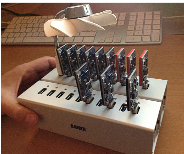
Figure 6: A USB hub hosting an array of ASICMINER Block Erupter USB-stick style bitcoin miners, and a USB-powered cooling fan. Each USB-stick uses a 130-nm ASIC that hashes at 330 MH/s, or about half the performance of $450 28-nm AMD 7970 GPU. Photo Credit: DennisD7.
