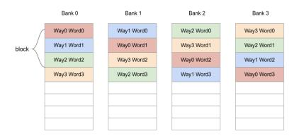
Figure 14: Block Interleaving Scheme
