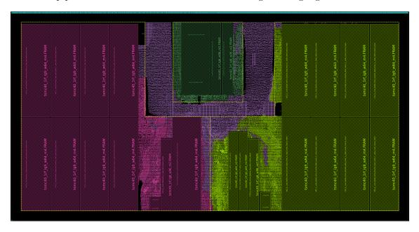
Figure 19: Single-core BlackParrot Floorplan (32 KB I-Cache, 32 KB D-Cache) (1250 um x 655 um) (TSMC 40 nm) (By courtesy of Chun Zhao)
