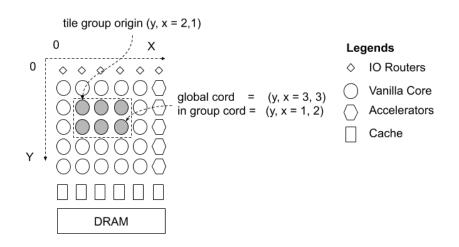
Figure 2: Top-level Manycore Diagram
