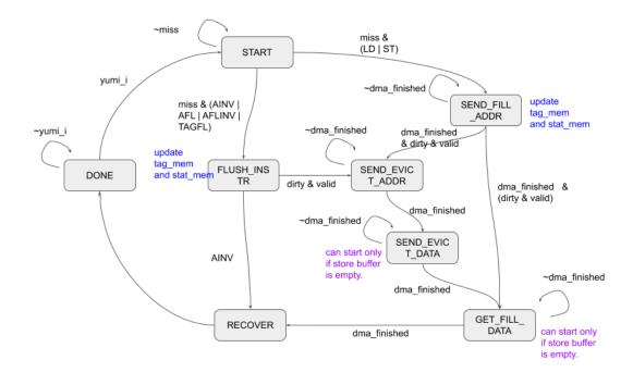
Figure 8: Miss handler Finite state machine
