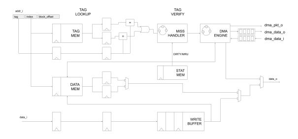
Figure 7: Victim cache high-level schematic
