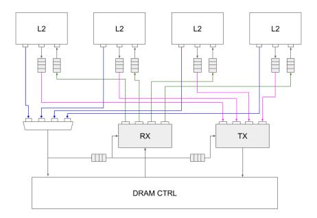
Figure 10: L2 DMA Interface Converter. RX/TX Abstraction. Blue line is for request. Pink line is for evict data. Green is for refill data.
