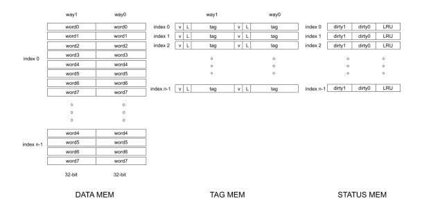
Figure 6: L2 Cache SRAM layout
