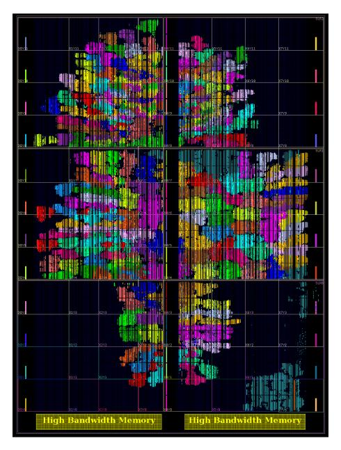
Figure 17: 12x12 Manycore on Xilinx VCU128 board (XCVU37P) (By courtesy of Leonard Xiang)
