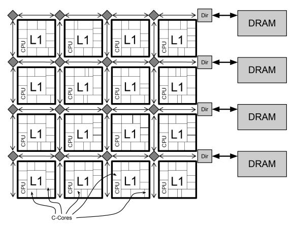
Figure 2.1: A Floorplan for GreenDroid with Directory Coherence In the cache-coherent GreenDroid prototype, directories sit between the MDN and DRAMs. Each tile includes a host CPU, L1 data and instruction caches, and a set of c-cores. The set of c-cores on each tile may be different, necessitating a mechanism for migrating execution between tiles.
