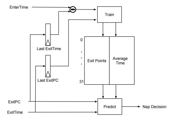
**Figure 4.1**: **The Idleness Predictor** When a tile exits – i.e. execution migrates to another tile – the local nap controller predicts whether the tile will be idle for long enough to merit napping.
