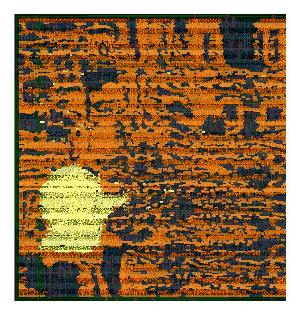
Figure 3.6: MCF 2006 conservation core for primal\_bea\_mpp() function The C-Core synthesizes to  $0.077mm^2$ , operates at speeds up to 1412 MHz, and provides 53% coverage for the application. The light gray elements are datapath logic (adders, comparators, etc.), dark gray elements are registers, and the white elements constitute the control path.
