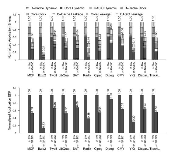
Figure 5.19: Quasi-ASIC enabled System Energy Efficiency The graphs show the energy and EDP reductions that QASICs provide compared to an inorder, power efficient MIPS core ("SW"). Results are normalized to running on the MIPS core (lower is better). The QASICs can reduce the application energy consumption and energy-delay product by up to 79% and 83% respectively.
