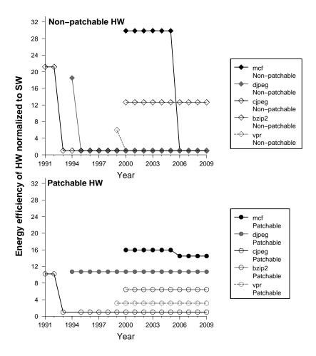
Figure 3.7: Conservation core effectiveness over time The patchable c-cores are able to support changes in code across versions of stable applications, enabling them to deliver efficiency gains over a very long period of time.
