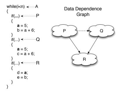
Figure 5.8: **Inferred Dependence Example** The solid and dashed lines show true and inferred dependences. There is an inferred dependence edge from P to Q because no valid ordering of P, Q, R orders Q before P (Section 5.2.4).
