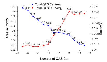
Figure 5.17: Impact of generalization on Qasic Area and Energy Efficiency for the Benchmark Set The labels on the area and energy curves show the ratio of area and energy requirements of the QASIC set compared to that of fully-specialized circuits.
