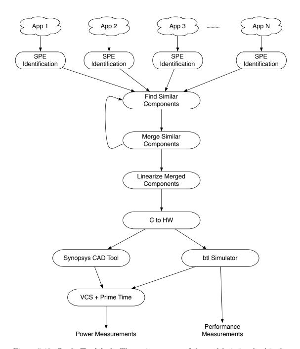
Figure 5.10: **Qasic Toolchain** The various stages of the toolchain involved in designing QASICs, generating the hardware for QASICs, as well as measuring QASIC's performance and power efficiency are shown.
