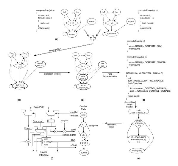
Figure 5.6: **Quasi-Architecture Example** An example showing the different stages involved in conversion of source code segments, computeSum and computePower (a) to QASIC hardware (f). The resultant QASIC can perform the functionality of the two input code segments as well as other functions like  $n!, c^{2^n}$ . The solid lines represent the control dependence and the dashed lines represent the data dependence for the program dependence graphs ((a), (b),(c)).
