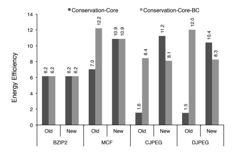
Figure 3.12: Improvements in the backward compatibility of Conservation Cores The energy-efficiency of the older versions improves significantly (up to  $7\times$ ) with minimal impact on that of newer ones.
