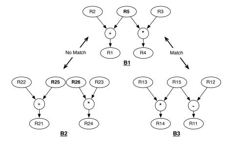
Figure 3.3: **Basic block matching** Target block B3 can be mapped onto the hardware for original block B1, but target block B2 does not match B1 and cannot be mapped: There is no consistent mapping between the register names in bold.
