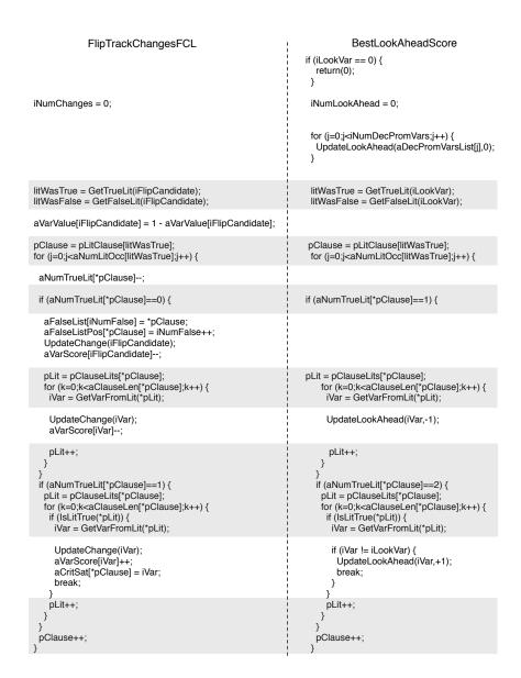
Figure 5.2: Similar code patterns present across the hotspots of a Sat Solver tool Figure highlights the similar code patterns that are present across the hotspots in UBC Sat Solver tool.
