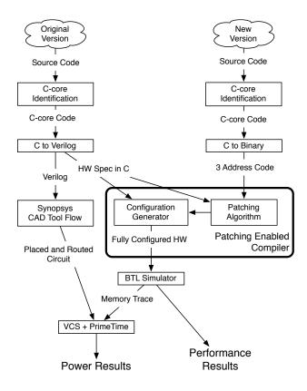
Figure 3.4: **The Patching Algorithm Toolchain** The various stages of our toolchain involved in hardware generation, patching, simulation, and power measurement are shown. The bold box contains the patch generation infrastructure based on our patching enabled compiler.
