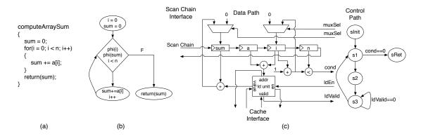
Figure 2.4: **Specialized Core Design Example** An example showing the translation from C code (a), to the compiler's internal representation (b), and finally to hardware (c). The hardware schematic and state machine correspond very closely to the data and control flow graphs of the C code.
