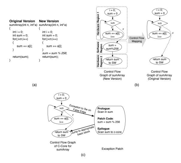
Figure 3.2: **Handling changes in control flow across versions** (a) The original and new source for sumArray() is shown. (b) The mapping between the new and the original version of sumArray's CFG covers most of the target version in two hardware regions. (c) Transfers of control between the hardware and software regions require an exception.
